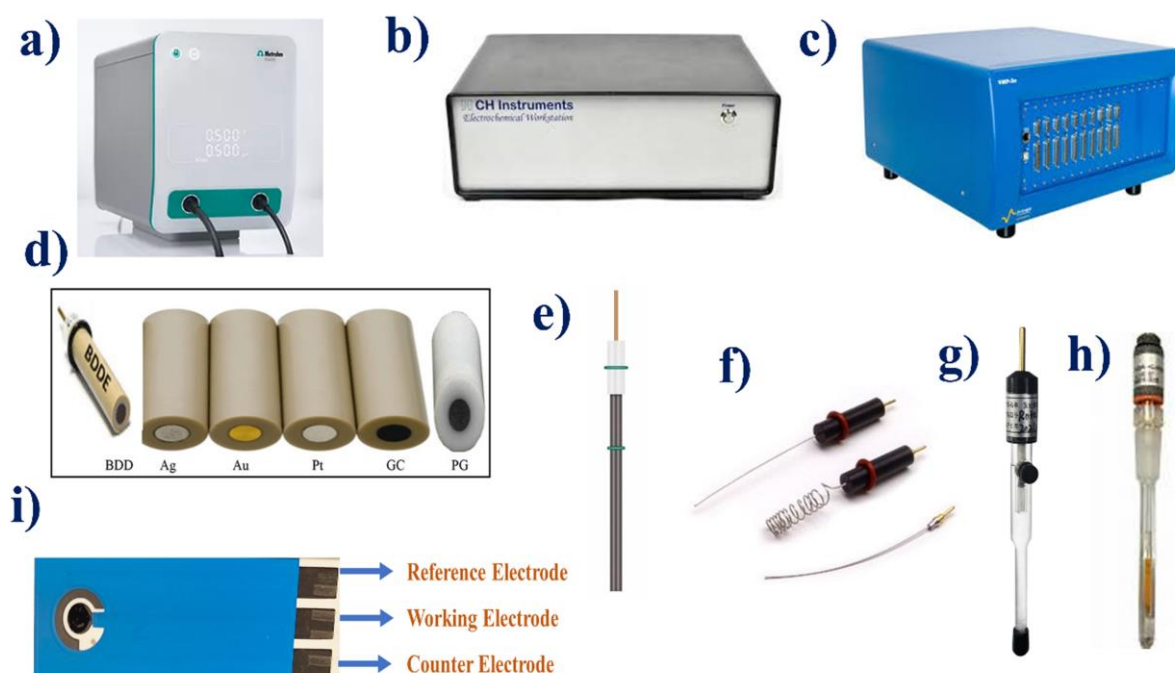
Figure 2. (a) Metrohm Autolab Potentiostat/Galvanostat (b) CHI Instrument Potentiostat (c) Biologic Potentiostat, (d) Working Electrode, (e) Graphite Counter Electrode, (f) Platinum Counter Electrode, (g) Ag/AgCl Reference Electrode (h) Hg/HgO Reference Electrode (i) Screen-Printed Electrode.
